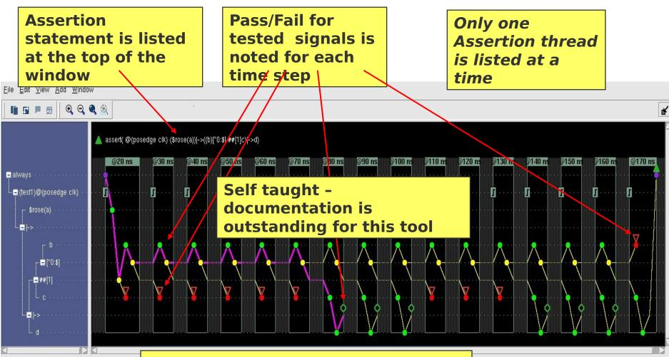
ATV must be enabled for a given assertion and a specific thread of that assertion prior to running a simulation
